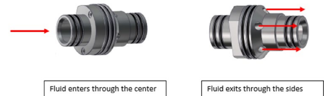
Figure 3 – Flow guide to divert the flow from inside the coiled tubing to outside on the camera lens
