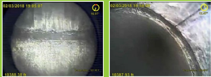
Figure 5C Figure 5D Figure 5B – Partially broken ceramic disc Figures 5C and 5D – Casing Collar texture observed, indicating liner exposed behind a potential parted pipe
