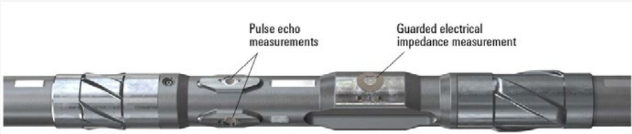
Figure 1: The new-generation dual-image OBM environment LWD imaging tool. The sensors send the pulses through the drilling fluid using the electromagnetic subsystem. These pulses are then sent into the formations at a wide range of frequencies to produce the resistivity images of the subsurface geological structures of the formations. The short ultrasonic pulses taken from the formations affected by the OBM are removed by the acoustic subsystem of the sensors. Combining both features helps make the new LWD imaging tool capable of recording high-resolution resistivity and ultrasonic images. The continuous sensors' sampling of the LWD tool of the ultrasonic and resistivity images improves the resolution of the produced images to surpass the images recorded by wireline tools1.
