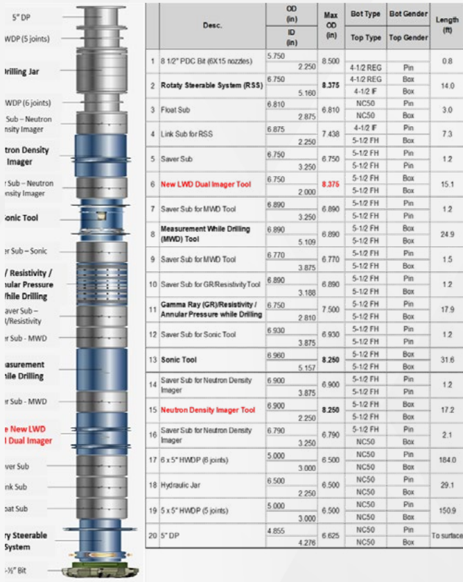
Figure 2: The LWD BHA configuration, including the new LWD OBM dual imager, while drilling with OBM in the wellbore.
