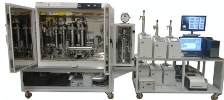
Figure 1. illustrates a generic core-flooding system consisting of a core holder inside an oven, with several pressure transducers and gauges, along with several pumps and a system to control and collect the pressure measurements.
